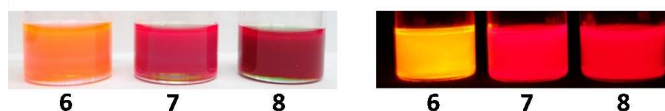
Fig. 2 Photographs of toluene solutions of 6-8 under ambient light (left) and under illumination of 365 nm light (right). The fluorescence of 6-8 is substantial even under ambient light, so that the solutions look cloudy (left).
