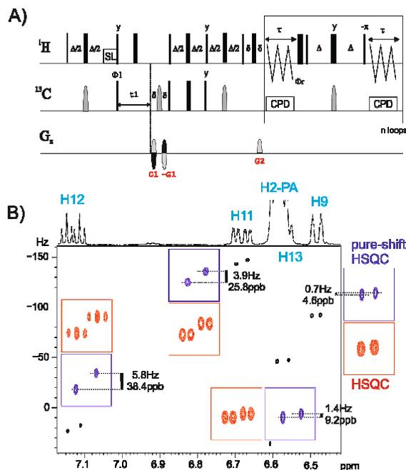
Figure 2: A) Pulse scheme of the pure shift sensitivity-improved HSQC experiment ( $\Delta = 1/(2 \cdot ^1\text{J}(\text{CH}))$ ); B) Expanded areas comparing some cross-peaks in SA- (red) and SAPS-HSQC (blue) spectra of the racemic compound **1**/R-PA mixture acquired with a reduced  $^{13}\text{C}$  spectral width of 2.5 ppm.
