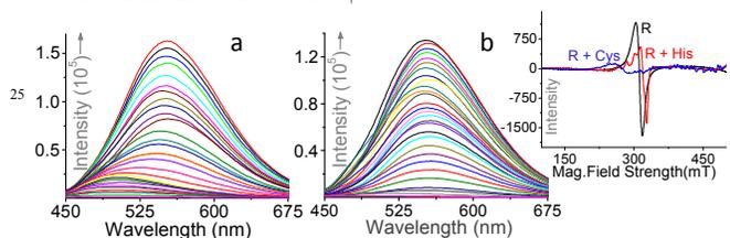
**Fig. 2** Changes in luminescence spectra for **R** (20  $\mu\text{M}$ ) in presence of varying (a)  $[\text{Cys}]$  (0 -  $2.8 \times 10^{-3}$  M) and (b)  $[\text{His}]$  (0 -  $3.2 \times 10^{-3}$  M) using  $\lambda_{\text{Ext}} = 350$  nm and slit width 3/3 nm; Inset: X-Band EPR spectrum of probe **R** (1.0 mM) in absence and presence of  $[\text{Cys}]$  (3.0 mM) and His (3.0 mM). All studies were performed in aq.-HEPES buffer (10 mM, pH 7.4) medium at 298K.
