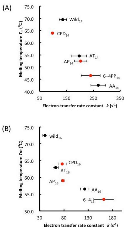
**Figure 2.** Summary of  $T_m$  against  $k$  plots for a series of (A) 14-mer and (B) 16-mer ds-DNAs. The  $T_m$  values were obtained by use of **1** and **2**. Probes **Fc1** and **Fc2** were used for the determination of  $k$  values that were based on three measurements. Error bars indicate the standard deviation (SD).
