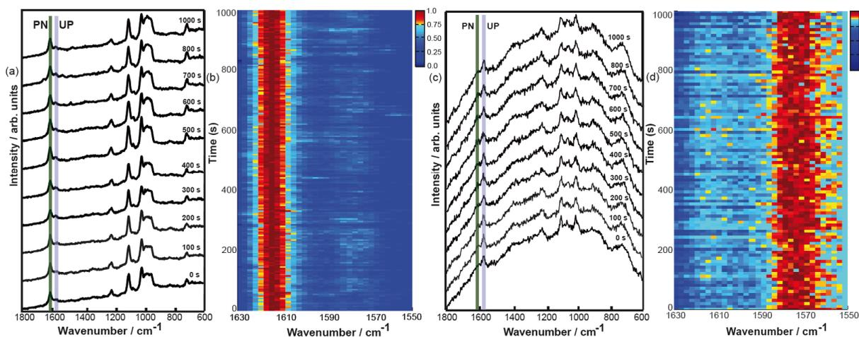
Fig 4 (a) Time-dependent TERS spectra of 4-MPY under ambient conditions (excitation 532nm /  $650\mu\text{W}$ ; integration time 5 s) (b) Colour coded intensity plot of the data (a) wavenumbers range from  $1550\text{-}1630\text{ cm}^{-1}$  (c) Time-dependent TERS spectra of 4-MPY under argon (excitation 532nm /  $650\mu\text{W}$ ; integration time 10 s). (d) TERS intensity plot of the data in (c) wavenumbers range from  $1550\text{-}1630\text{ cm}^{-1}$ .
