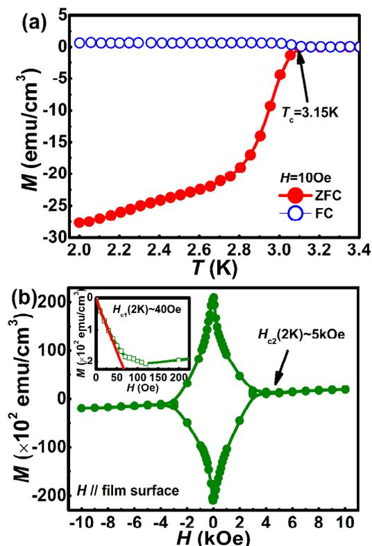
**Fig. 4** (a) Temperature dependence of magnetism with FC and ZFC modes under 10 Oe applied magnetic field parallel to the surface; (b)  $M(H)$  loop at 2 K and the inset is the low-field  $M(H)$  to give the  $H_{c1}$  at 2 K.
