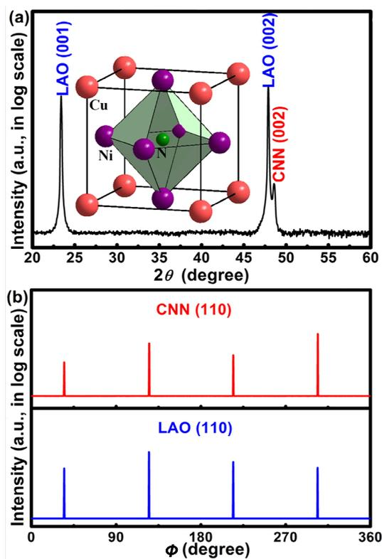
**Fig. 1** (a) XRD  $\theta$ - $2\theta$  result of CNN film on LAO (001) and the inset shows the crystal structure of CNN; (b) XRD  $\phi$ -scans from (110) reflections of CNN and LAO.
