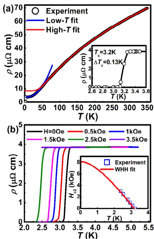
**Fig. 3** (a) Temperature dependence of resistivity of the CNN film on LAO (001) under a zero field as well as the transport fitting results and the inset is the enlarged image to give a clear superconducting transition; (b) superconducting transition under different magnetic fields and the inset is the fitting result by the WHH expression.
