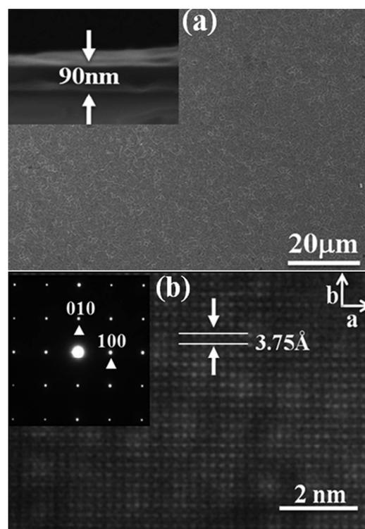
**Fig. 2** (a) Surface FE-SEM result of CNN/LAO and the inset gives the thickness about 90 nm; (b) surface HRTEM result of the CNN film and the inset is the SAED.
