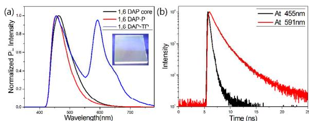
**Fig. 1** (a) Normalized PL spectra of the compounds (vacuum-deposited film on glass, inset: 1,6 DAP-TP film); (b) Time-resolved emission decays obtained from the vacuum-deposited 1,6 DAP-TP films.
