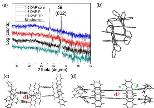
**Fig. 2** (a) Out-of-plane XRD patterns obtained from the 1,6 DAP core, 1,6 DAP-P, and 1,6 DAP-TP (200 nm films deposited on Si substrates); (b) side view of the 1,6 DAP-TP dimer structure; (c) pyrene top view of the 1,6 DAP-TP dimer structure; (d) anthracene top view of the 1,6 DAP-TP dimer structure (calculated at the  $\omega$ B97XD/6-31G(d) level of theory).
