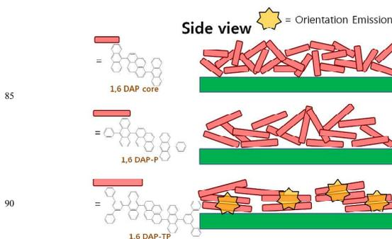
**Fig. 3** Schematic diagram showing the stacking structures of the synthesized compounds.
