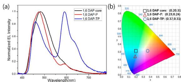
**Fig. 4** (a) Normalized EL spectra, (b) CIE chromaticity diagram of the synthesized compounds using an emitting layer in the OLED device, yielding 10 mA/cm<sup>2</sup>.
