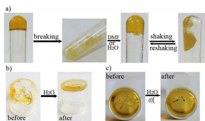
Fig. 4 (a) The solvent-healed and deformation recovery process of the broken gel 1 (4 %, 1 mL DMF), (b) the large area damage of gel 1 (3 %, 0.5 mL DMF) was repaired by adding H 2 O (0.25 mL), (c) the sonication-assisted healable process of a cross rupture.
