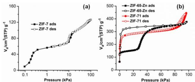
Figure 4 (a), adsorption-desorption isotherms of CO<sub>2</sub> on ZIF-7 at 195K; (b), adsorption-desorption isotherms of N<sub>2</sub> on ZIF-65-Zn (black) and ZIF-71 (red) at 77K.
