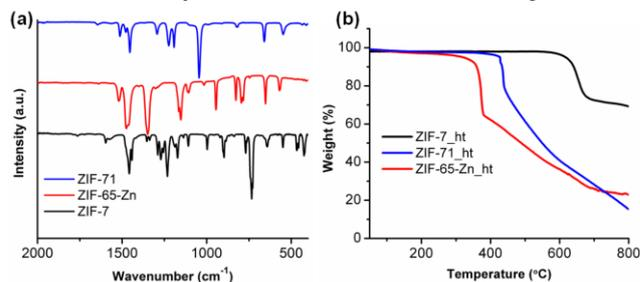
Figure 3 IR spectra (a) and TGA curves (b) of activated ZIF-7, ZIF-65-Zn and ZIF-71.
