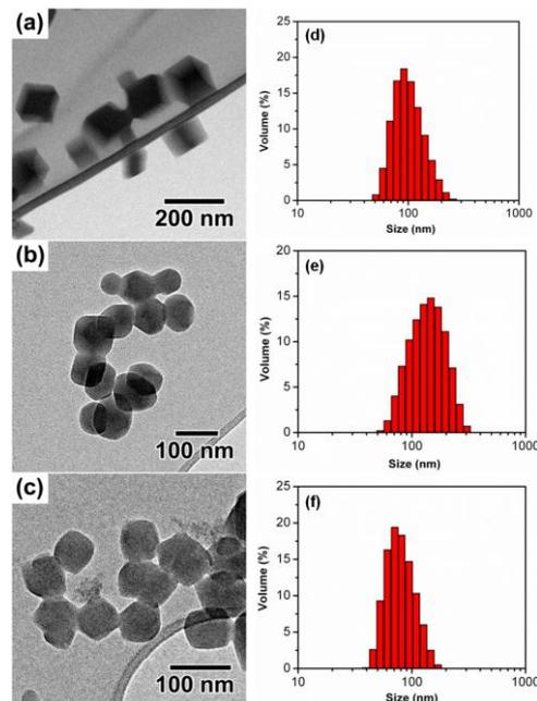
Figure 2 BFTEM images of nanosized ZIF-7 (a), ZIF-65-Zn(b), ZIF-71(c) and particle size distribution of ZIF-7 (d), ZIF-65-Zn(e), ZIF-71(f) by DLS measurements at room temperature.
