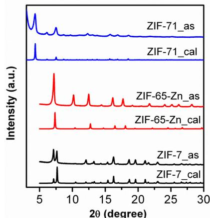
Figure 1 PXRD patterns of as-synthesized ZIF-7, ZIF-65-Zn and ZIF-71 in comparison with corresponding calculated patterns.
