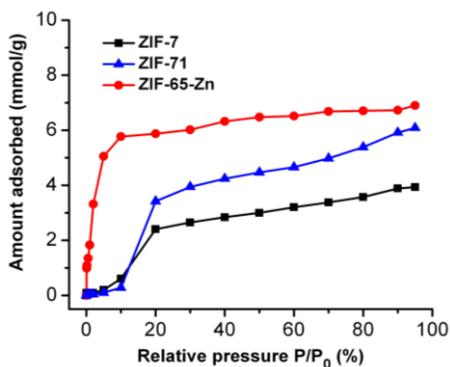
Figure 5 Vapor phase adsorption isotherms of methanol on ZIF-7, ZIF-65-Zn and ZIF-71 coated QCM substrates at 293K. The saturated vapor pressure P<sub>0</sub> of methanol at 293K is 12.98kPa.
