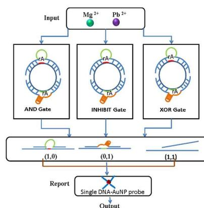
Fig. 13 AND, INHIBIT, and XOR logic gates connected to single DNAa-b-AuNP probes as colorimetric outputs. Each path is characterized by colorimetric and UV/Vis detection. Reproduced with permission from ref. 145. Copyright 2010 Wiley-VCH.
