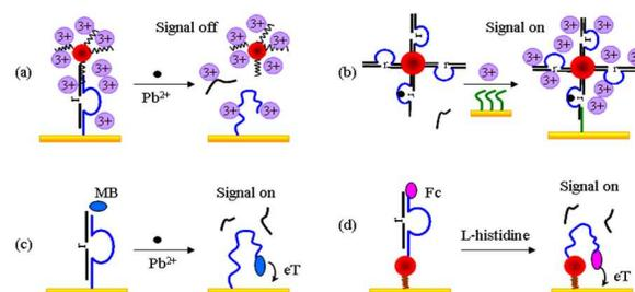
Fig. 6 (a) and (b) Schematic illustration of electrochemical biosensors for  $\text{Pb}^{2+}$  based on DNAzyme using DNA-Au bioconjugates as bio-bar codes to amplify the electrochemical signals from  $\text{Ru}(\text{NH}_3)_6^{3+}$ . The design was a “signal off” type biosensor in (a) and “signal on” type biosensor in (b). (c) and (d) Schematic illustration of conformation switch “signal on” electrochemical biosensors for (c)  $\text{Pb}^{2+}$  and (d) L-histidine.
