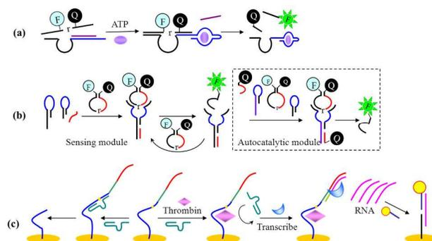
Fig. 8 (a) Structure-switching DNAzyme based fluorescent probe for ATP detection. (b) Amplified detection of DNA through an autocatalytic and catabolic DNAzyme-mediated process. (c) DNAzyme footprinting methodology using protein-aptamer complexes to block the DNAzyme cleavage activity. Subsequent surface RNA transcription and nanoparticle-enhanced SPR imaging was carried out for the detection.
