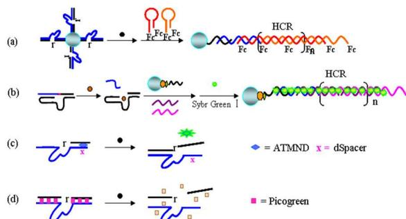
Fig. 7 Enzyme and nanoparticles free signal amplification methods for DNAzyme-based biosensors. (a) (b) Using hybridization chain reaction (HCR). (c) Using a dSpacer that can bind an extrinsic fluorescent compound and quench its fluorescence. (d) Using double-strand-chelating dye Picogreen (PG).
