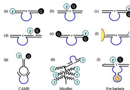
Fig. 2 Schematic illustration of the arrangement of fluorophore/quencher (F/Q) pairs on the DNAzyme. (a) F and Q were placed at the two ends of the substrate strands. (b) F and Q were placed next to the cleavage site flanking the cleavage site. (c) F and Q were placed on the same side but different strands. (d) Use an extended enzyme part acting as a template to place the Q close to the F. (e) A second Q was introduced on the other end of the
