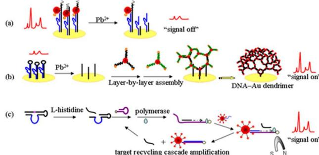
Fig. 5 Schematic design of SERS and DNAzyme based biosensor. (a) “Signal off” type biosensor for  $\text{Pb}^{2+}$  detection. (b) “Signal on” type biosensor using
