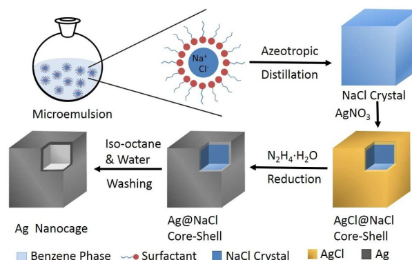
Scheme 1 Schematic illustration of the azeotropic distillation assisted (AD) route for the formation of Ag nanocage.
