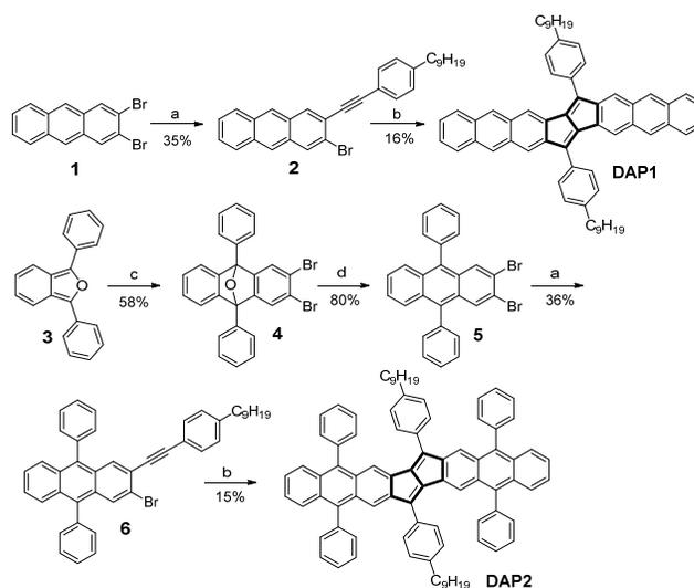
**Scheme 1** Synthetic route to DAP1 and DAP2. Reagents and conditions: (a) 1-ethynyl-4-nonylbenzene, Pd(PPh<sub>3</sub>)<sub>2</sub>Cl<sub>2</sub>, CuI, Et<sub>3</sub>N/THF, 75 °C, overnight; (b) Pd<sub>2</sub>(dba)<sub>3</sub>, P(2-furyl)<sub>3</sub>, Cs<sub>2</sub>CO<sub>3</sub>, CsF, hydroquinone, 1,4-dioxane, 135 °C, 36 h; (c) 1) 1,2,4,5-tetrabromobenzene, *n*-BuLi, toluene, -50 °C, 2) RT, overnight; (d) Zn, TiCl<sub>4</sub>, THF, 0-70 °C, reflux overnight.
