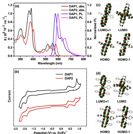
**Fig. 1** (a) UV-vis absorption and photoluminescence (PL) spectra of **DAP1** and **DAP2** in chloroform; (b) Cyclic voltammograms of **DAP1** and **DAP2** recorded in dry dichloromethane; frontier molecular orbital profiles of **DAP1** (c) and **DAP2** (d) based on DFT (B3LYP/6-31G\*\*) calculations.
