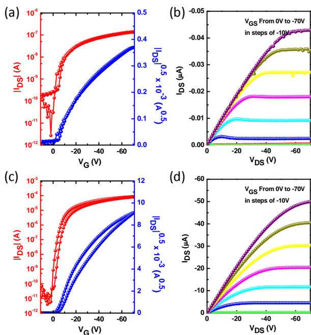
**Fig. 4** Transfer and output characteristics of **DAP1** (a, b) and **DAP2** (c, d) devices with ODTS treatment.
