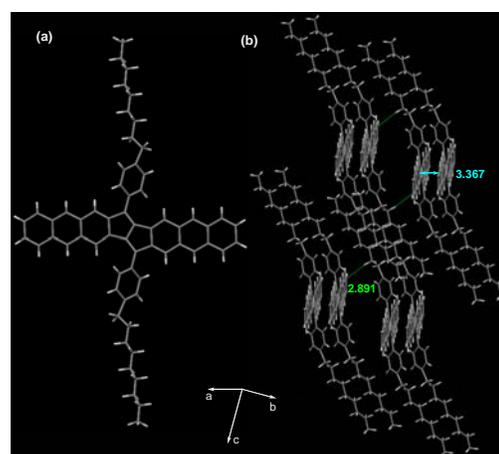
**Fig. 2** (a) Crystallographic structure of **DAP1**; (b) 3D packing structure of **DAP1**, showing intermolecular  $\pi$ - $\pi$  and [C-H... $\pi$ ] interactions.
