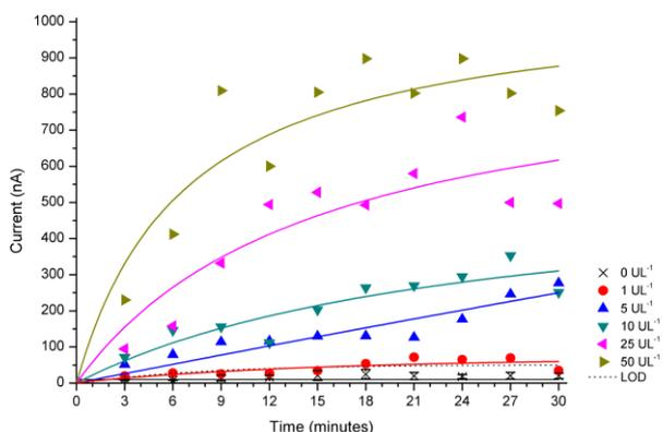
**Fig. 5** Amperometric response of ferrocenylamine released from substrate 1 (50  $\mu\text{M}$ ) after the addition of ALP in different concentrations. Error bars indicate standard deviations ( $n = 3$ ). LOD calculated as  $3 \times$  standard deviations higher than the mean.
