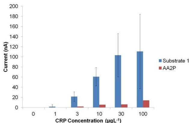
**Fig. 7** Current measured from CRP ELISA using substrate **1** and AA2P as electrochemical. Error bars indicate standard deviations ( $n = 6$ ).
