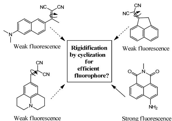
**Scheme 1:** comparison of the structures of three Knoevenagel adducts with weak fluorescence and that of strong fluorescent 4-amino 1,8 naphthalimide indicating the strategy to get efficient fluorophores
