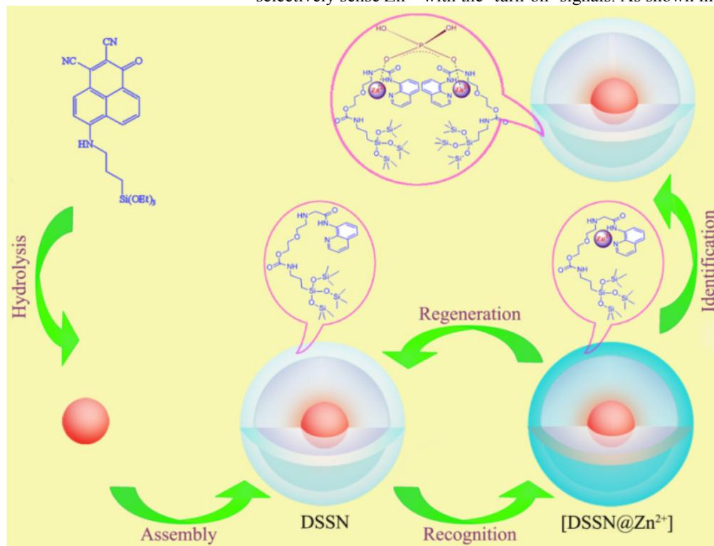
**Figure 1:** the structure of a siloxane-modified fluorophore and the design concept of nanoparticle-based ratiometric chemosensors for  $Zn^{2+}$  and  $H_2PO_4^-$
