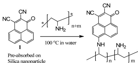
**Scheme 10:** the synthesis strategy of polymer-silica hybrid fluorescent particle by nucleophilic aromatic substitution of **1** adsorbed onto silica particles
