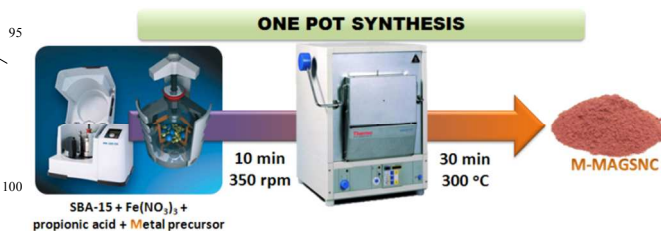
Scheme 3. Overview of the preparation of functionalized magnetic nanocomposites.
