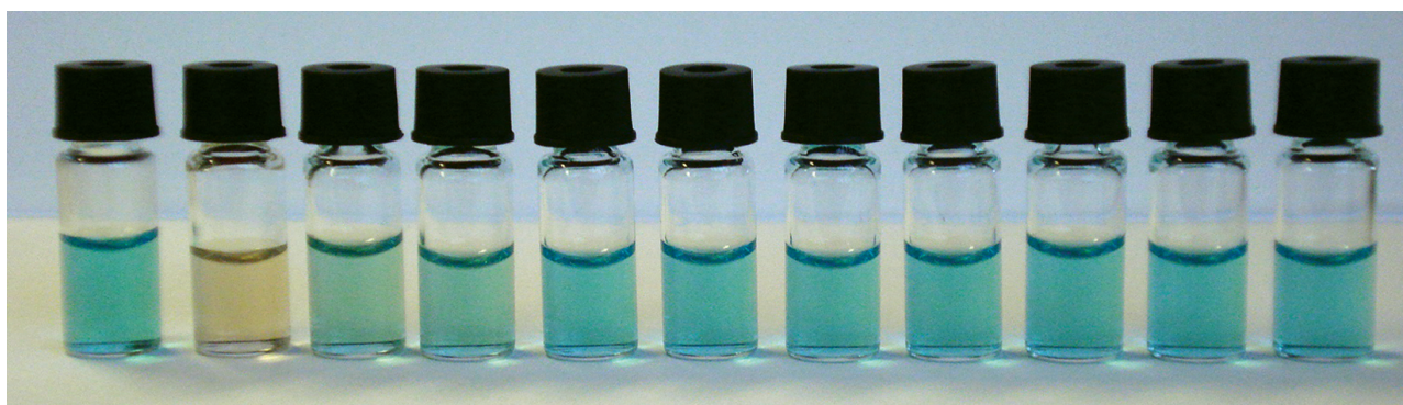
Figure 13. The colours of the 1 : 1 mixtures of 71 : PV ( 20 \mu\text{M} each) with and without anions (sodium salts) from left to right: no anion, PPI, ATP, ADP, AMP, c-AMP, phosphothreonine, phosphoserine, phosphotyrosine, \text{HPO}_4^{2-} and citrate (5 equiv. each).
