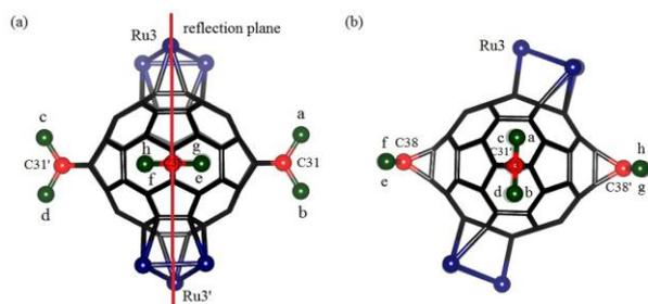
**Fig. 4** (a) Front and (b) side views of the *parallel-3* isomer. The ethyl formate groups ( $\text{COOC}_2\text{H}_5$ ) are denoted by green balls and the  $\text{Ru}(\text{CO})_3$  groups are denoted by blue balls.
