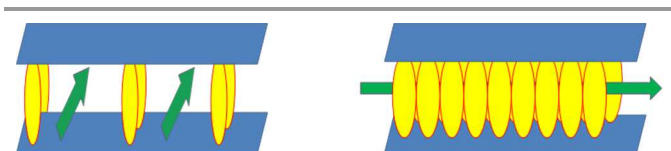
Fig 2. Diagram of 1-directionality of the channels within the hydrogen bonded framework where the guest molecules reside
