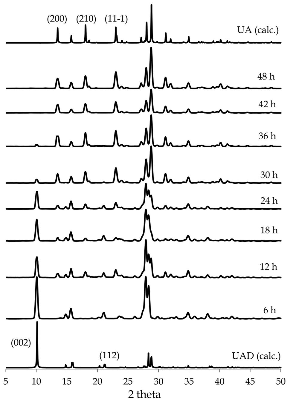
**Fig. 3.** PXRD patterns of the transformation of UAD to UA in pH 4 McIlvaine buffer at 37° C. The diffraction pattern at 6 h showed reflections corresponding mostly to UAD. At 12-36 h, both UAD and UA were present. By 42-48 h, diffraction lines corresponded exclusively to UA, indicating that the transformation was complete.
