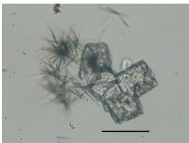
**Fig. 5.** Photomicrograph of the transformation of UAD in pH 6.8 McIlvaine buffer at 37° C, taken after 42 hours. Scale bar = 100  $\mu\text{m}$ .
