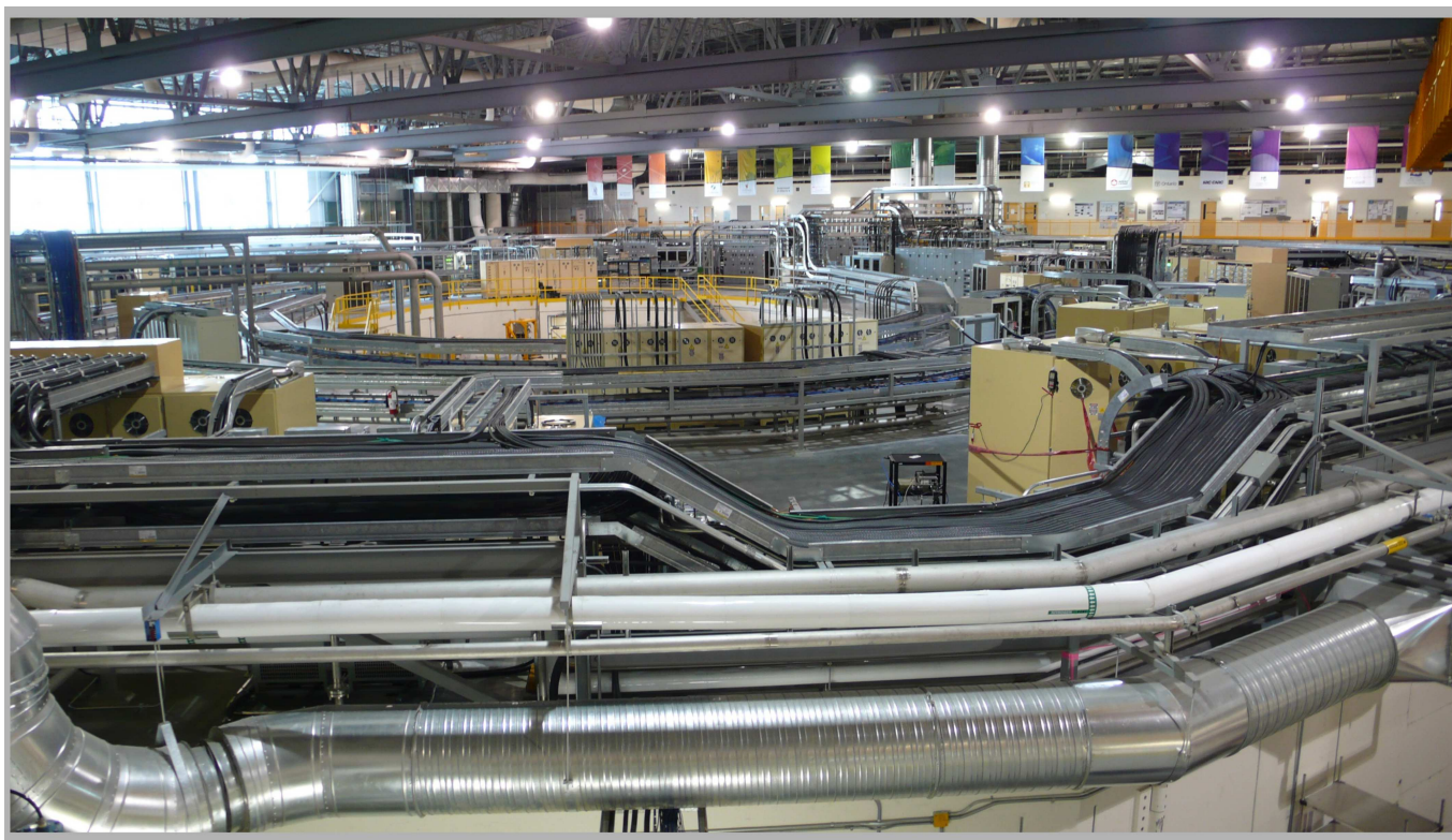
FIG. 15: At the core of the Canadian Light Source are three particle accelerators: an electron linear accelerator (located underground), a booster synchrotron (the inner ring in this photo) and an electron storage ring (hidden in the foreground). The electron storage ring operates at a current of 250 mA with an energy of 2.9 GeV. The long stored beam lifetime has permitted electron re-injection to be reduced to twice per day. The storage ring, with a 171 meter circumference, supports 14 independent beam lines from THz region (about 0.025 eV) to hard X-rays (more than 100 keV).
