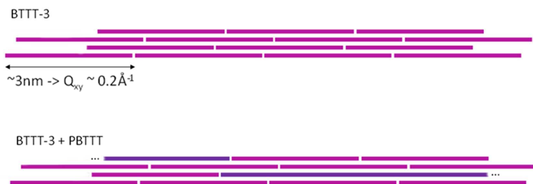
Figure 4. Cartoon of the proposed mixing of BTTT-3 and PBTTT chains within crystallites.
