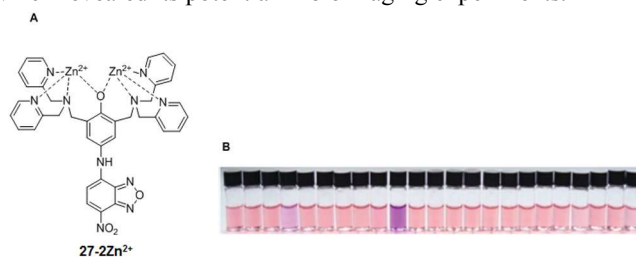
Fig. 16. A) Sensor 27-2Zn 2+ . B) Colour changes of sensor 27-2Zn 2+ in 50 mM aqueous HEPES buffer solution (pH 7.4), [ 27-2Zn 2+ ] = 35 μM, [other anions] = 175 μM. Anions from left to right: none, AMP, ADP, ATP, PO 4 3- , H 2 PO 4 - , PhPi, NPhPi, PPI, F - , Cl - , Br - , I - , NO 3 - , SO 4 2- , HCO 3 - , CH 3 CO 2 - , citrate, N 3 - , ClO 4 - , S 2 O 7 2- , C 2 O 4 2- .
