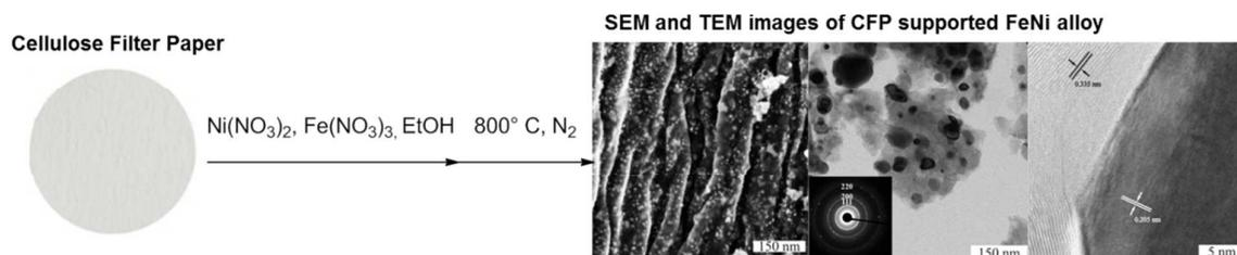
**Figure 4.** Schematic representation of carbon supported FeNi nanoparticles obtained by carbothermal reduction of cellulose. Figure adapted from ref 25, © 2014.
