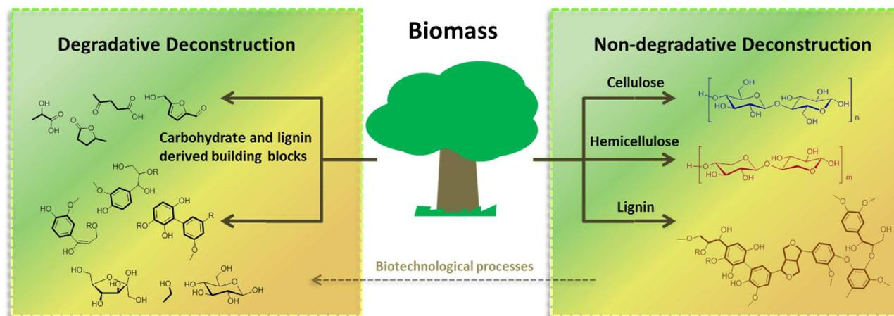
**Figure 2.** A representation of degradative (DD) and non-degradative (NDD) deconstruction processes, for the valorization of biomass.
