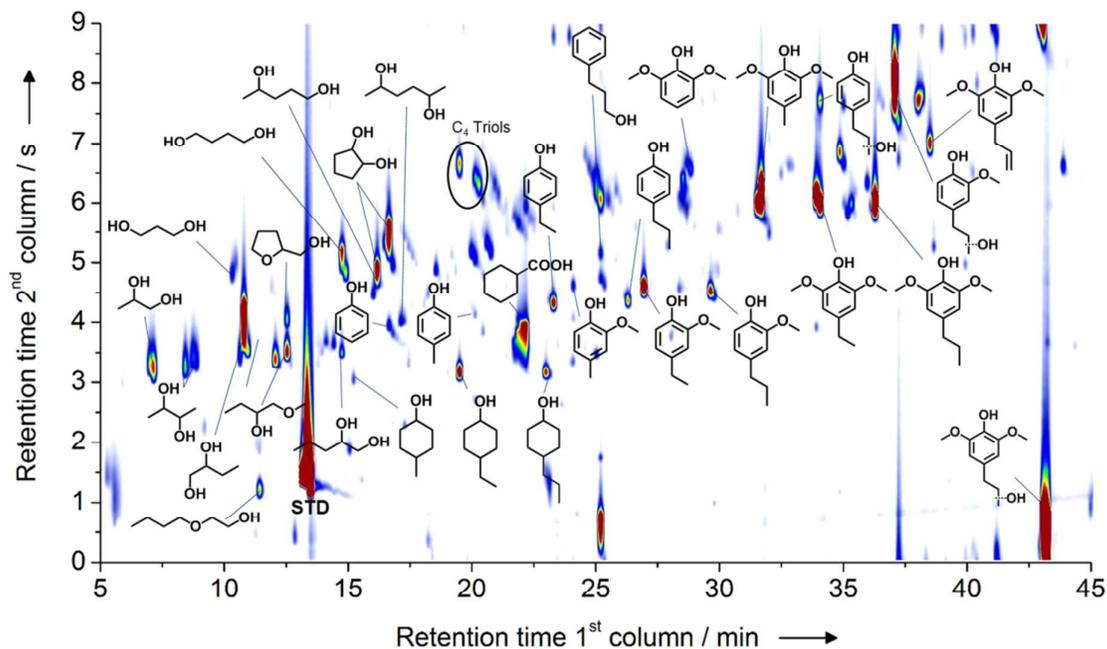
**Figure 7.** Speciation of the products obtained from the catalytic biorefining of poplar wood in the presence of Raney Ni at 180°C for 3 h (2-PrOH/H<sub>2</sub>O, 7:3, v/v). Reproduced with permission from ref. 35. Copyright 2014, Wiley-VCH Verlag GmbH & Co. KGaA, Weinheim.
