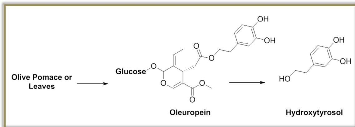
**Figure 10.** Schematic processing of vegetable residues for the extraction of Hydroxytyrosol.
