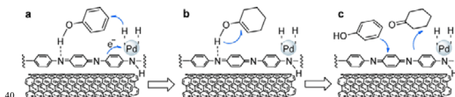
Fig 7. Proposed mechanism of the selective hydrogenation of phenol over Pd-PANI/CNT. Reproduced with permission from Ref. 31. Copyright © 2013 WILEY-VCH Verlag GmbH & Co. KGaA, Weinheim.
