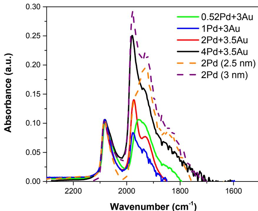
**Figure 4: DRIFTS spectra of the adsorption of carbon monoxide on silica supported PdAu catalysts: 0.52%Pd-3%Au (green), 1%Pd-3%Au (blue), 2%Pd-3.5%Au (red) and 4%Pd-3.5%Au (black) and monometallic Pd catalysts of similar particle size (dotted lines): 2.5 nm (orange) and 3 nm (purple). Intensity of linear bound CO peak at 2082  $\text{cm}^{-1}$  normalized for each catalyst for comparison.**
