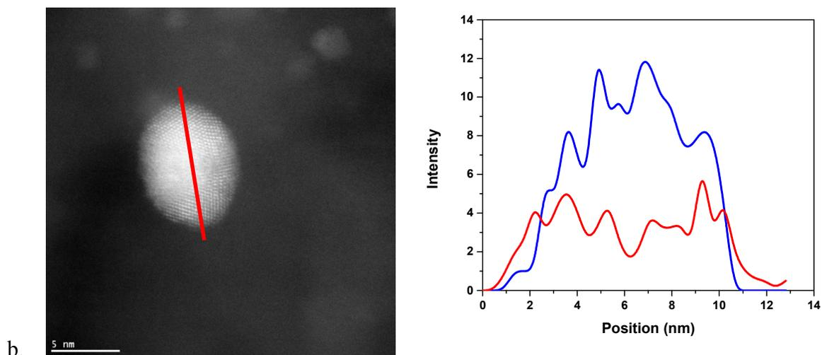
**Figure 2: Linescan data for 0.52%Pd-3%Au catalyst (a) and 1%Pd-3%Au catalyst (b) Pd (red) and Au (blue).**
