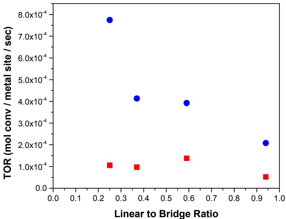
**Figure 6: Hydrogenolysis (blue circles) and isomerization (red squares) turnover rate versus the linear to bridge ratio from DRIFTS of CO adsorption .**
