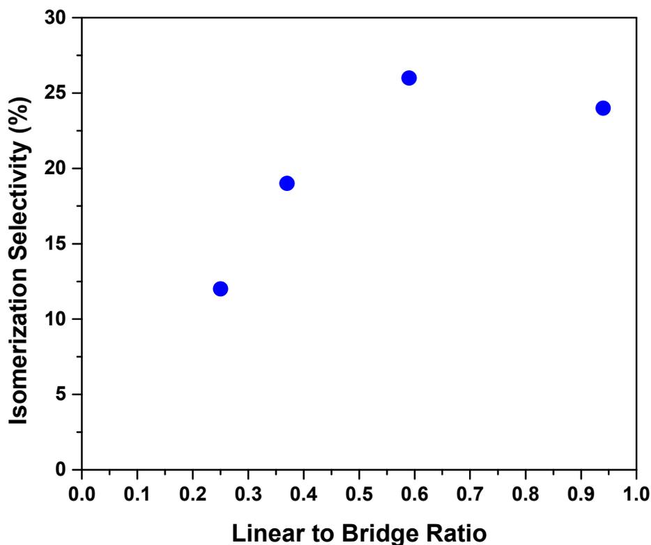
**Figure 7: Linear-to-Bridge ratio from DRIFTS of CO adsorption vs. Isomerization selectivity for PdAu catalysts**
