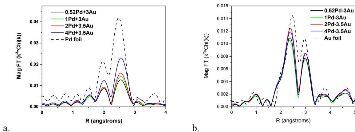
**Figure 3: EXAFS spectra for (a) Pd K-edge and (b) Au L<sub>3</sub>-edge**
