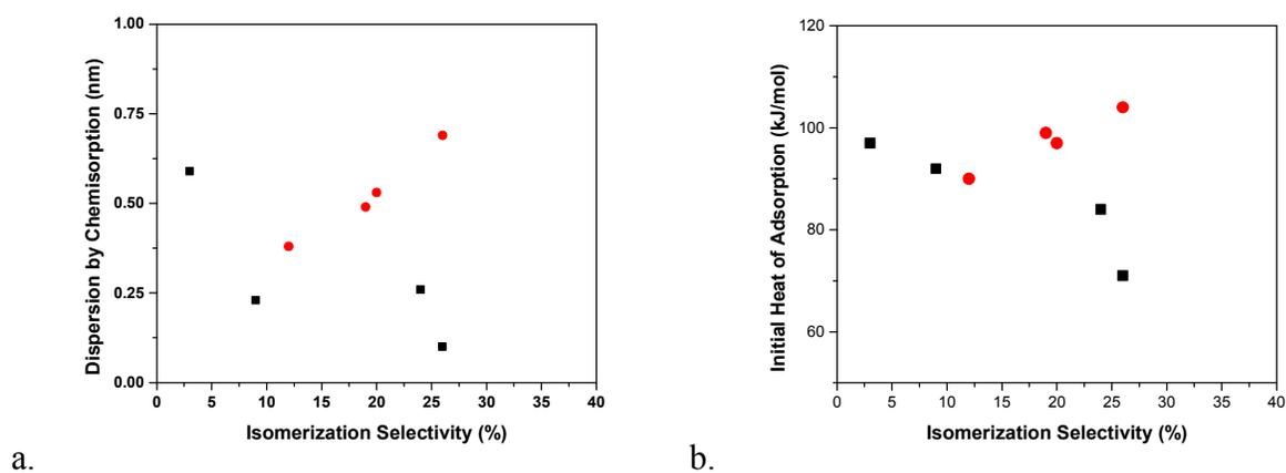
**Figure 5: a) Isomerization selectivity vs. Particle size determined by CO chemisorption and b) Initial CO heat of adsorption vs. Isomerization selectivity of monometallic Pd (black squares) and PdAu (red circles) catalysts**
