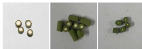
Fig.2. Pictures of different supports loading Cr. (1)Cr(8.56%)/ZnAlLaO; (2)Cr(18.12%)/ZnAlLaO; (3)Cr(32.03%)/ZnAlLaO
