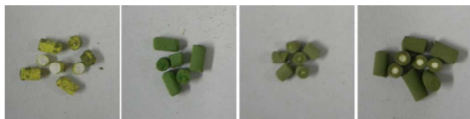
Fig.1. Pictures of different supports used for loading Cr. (a) Cr/CaAlLaO; (b) Cr/CrAlLaO; (c) Cr/MgAlLaO; (d) Cr/ZnAlLaO. Cr loading: 18 wt%
