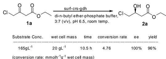
**Scheme 1** Designer cell catalysed production of ethyl (S)-4-chloro-3-hydroxybutyrate.
