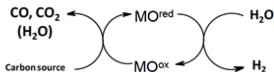
Scheme 1: Key principle of the chemical looping for H 2 production
