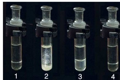
Fig. 2 Catalyst recycling and phase behaviour in DBT oxidation in heptane-water two-phase system catalysed by PIB-PW (for better presentation, the amount of aqueous phase increased five-fold): (1) initial reaction system with heptane phase (top) and aqueous H_2O_2 phase (bottom); (2) the system after first reaction run complete showing DBT sulfone white precipitate; (3) the system after second extraction with acetonitrile – heptane phase (top) and acetonitrile phase (bottom); (4) the system ready for second run with fresh amounts of DBT and aqueous H_2O_2 added.
