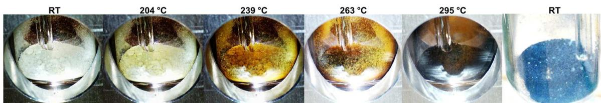
**Figure 6** Temperature programmed photographic analysis of  $\text{Y}(\text{BH}_4)_3$  (**s12\_Wdesolv**),  $\Delta T/\Delta t = 10$  °C/min,  $p(\text{Ar}) = 1$  bar.
