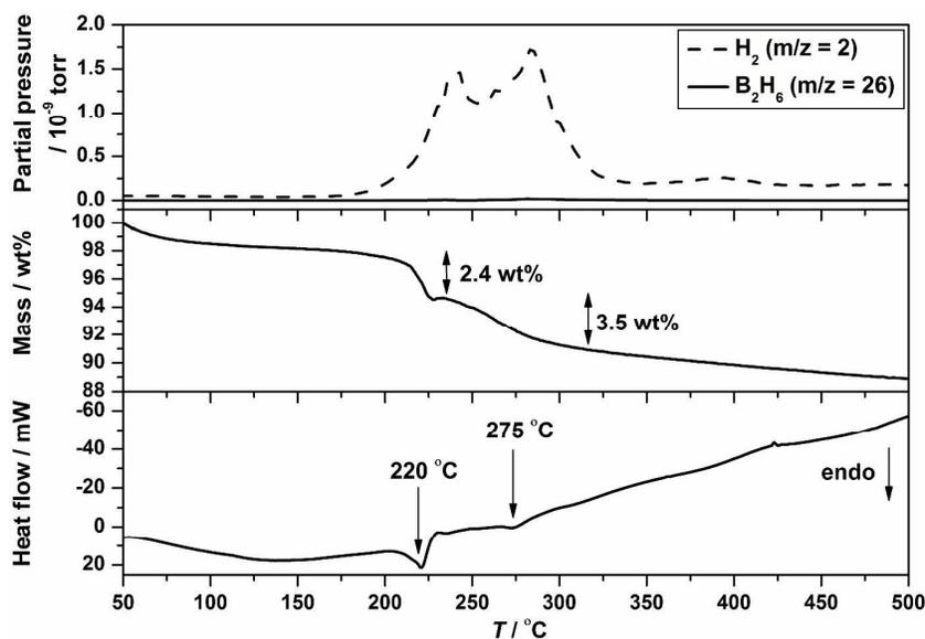
**Figure 9** Mass spectrometry (top), thermogravimetry (middle) and differential scanning calorimetry (bottom) of  $\text{Y}(\text{BH}_4)_3\text{-LiCl}$  1:1 (**s17**) in the temperature range 50 to 500  $^{\circ}\text{C}$ ,  $\Delta T/\Delta t = 10$   $^{\circ}\text{C}/\text{min}$ .
