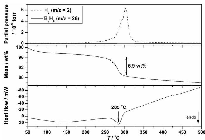
**Figure 5** Mass spectrometry (top), thermogravimetry (middle) and differential scanning calorimetry (bottom) of  $\text{Y}(\text{BH}_4)_3$  (**s12\_Wdesolv**) in the temperature range 50 to 500 °C,  $\Delta T/\Delta t = 5$  °C/min.
