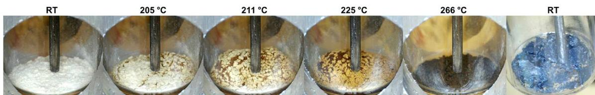
**Figure 10** Temperature programmed photographic analysis of  $\text{Y}(\text{BH}_4)_3\text{-LiCl}$  1:1 (**s17**),  $\Delta T/\Delta t = 10$  °C/min,  $p(\text{Ar}) = 1$  bar.
