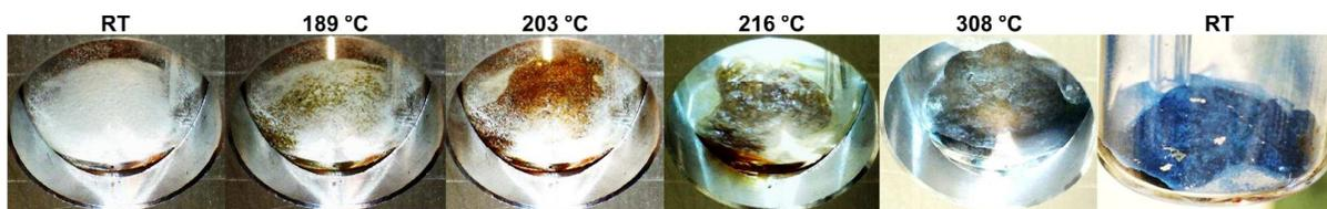
**Figure 8** Temperature programmed photographic analysis of  $\text{Y}(\text{BH}_4)_3\text{-LiBH}_4$  1:1 (**s16**),  $\Delta T/\Delta t = 10$   $^{\circ}\text{C}/\text{min}$ ,  $p(\text{Ar}) = 1$  bar.
