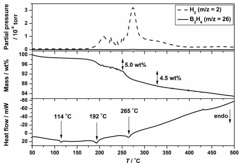
**Figure 7** Mass spectrometry (top), thermogravimetry (middle) and differential scanning calorimetry (bottom) of  $\text{Y}(\text{BH}_4)_3\text{-LiBH}_4$  1:1 (**s16**) in the temperature range 50 to 500  $^{\circ}\text{C}$ ,  $\Delta T/\Delta t = 10$   $^{\circ}\text{C}/\text{min}$ .
