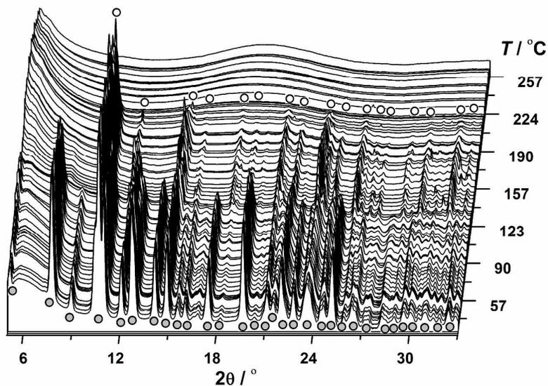
**Figure 4** *In situ* SR-PXD data for  $\text{Y}(\text{BH}_4)_3\text{S}(\text{CH}_3)_2$  (**s8\_Wsolv**) from RT to 260 °C,  $\Delta T/\Delta t = 3$  °C/min,  $p(\text{Ar}) = 1$  bar,  $\lambda = 1.020345$  Å. Symbols: Grey circle  $\text{Y}(\text{BH}_4)_3\text{S}(\text{CH}_3)_2$ , white circle  $\alpha\text{-Y}(\text{BH}_4)_3$ .
