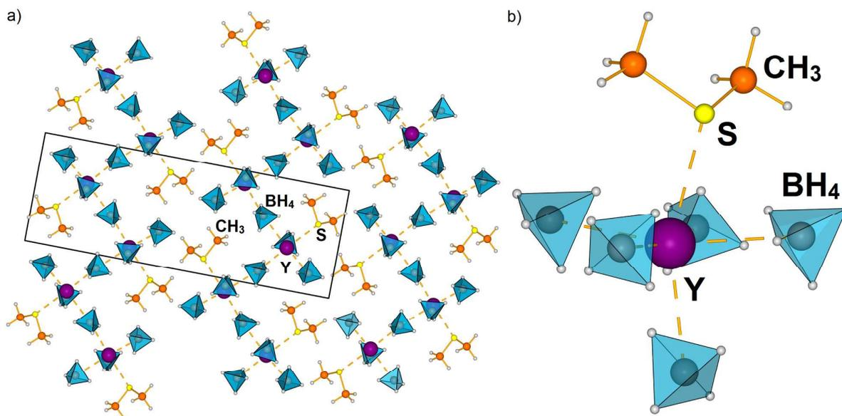
**Figure 2** a) Crystal structure of the novel solvate  $\text{Y}(\text{BH}_4)_3\text{S}(\text{CH}_3)_2$  composed of buckled layers of distorted octahedrons of 6-fold coordinated yttrium. The  $\text{BH}_4$  groups are shown as light blue tetrahedra and  $\text{Y}$  in purple. The  $\text{Y}-\text{B}$  and  $\text{Y}-\text{S}$  coordinations are shown as broken lines. b) Distorted octahedron of yttrium coordinated to five borohydride groups and one dimethyl sulfide group.
