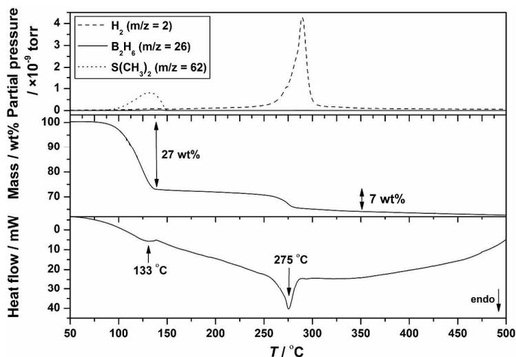
**Figure 3** Mass spectrometry (top), thermogravimetry (middle) and differential scanning calorimetry (bottom) of  $\text{Y}(\text{BH}_4)_3\text{S}(\text{CH}_3)_2$  (**s8\_Wsolv**) in the temperature range 50 to 500 °C,  $\Delta T/\Delta t = 5$  °C/min.
