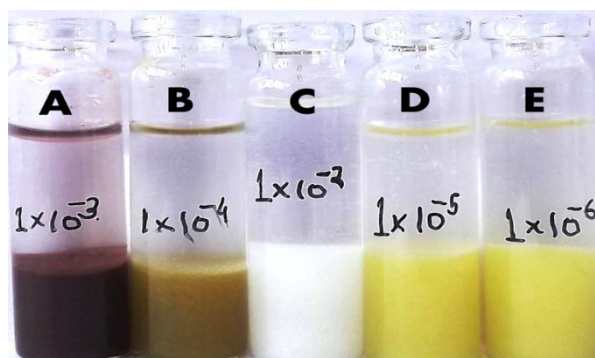
Fig. 6 Practical application of PPT-1 for detection of \text{Cu}^{2+} by silica support method.
