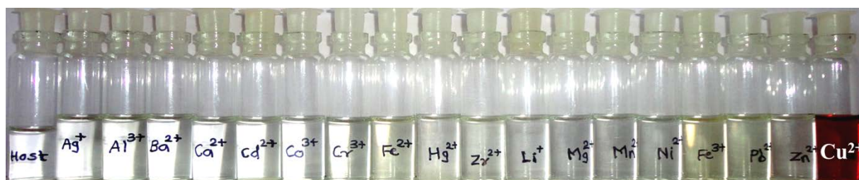
Fig. 1 Naked-eye detection of \text{Cu}^{2+} ion by PPT-1 in the presence of other metal cations under visible or sunlight.
