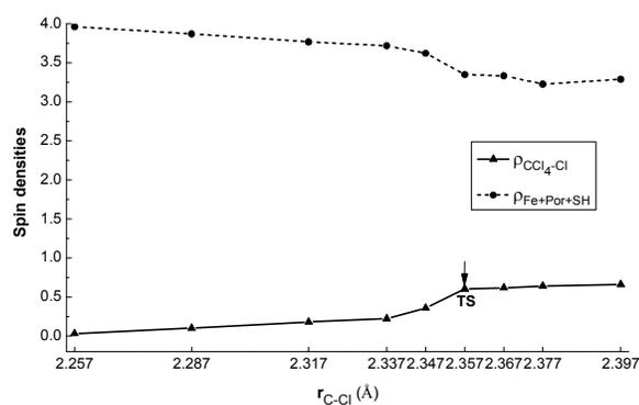
**Fig. 3** Changes in the spin densities ( $\rho$ ) on Iron+Porphine+Thiolate (Fe+Por+SH) and Substrate-Chloride ( $\text{CCl}_4\text{-Cl}$ ) moieties as a function of the C-Cl distance, which are calculated at the UB3LYP/B1 level in the gas-phase.
