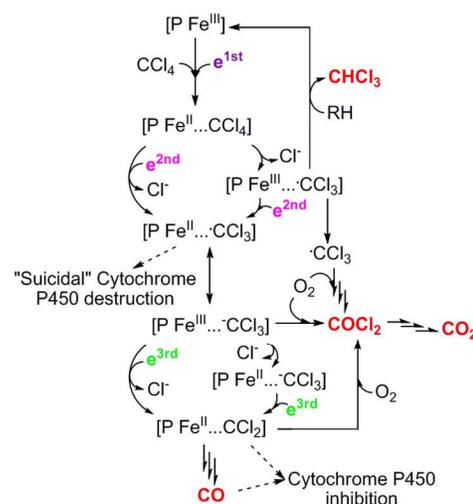
**Scheme 1.** Proposed mechanism for CCl<sub>4</sub> biotransformation by P450 enzymes and possible effect of metabolites on P450.
