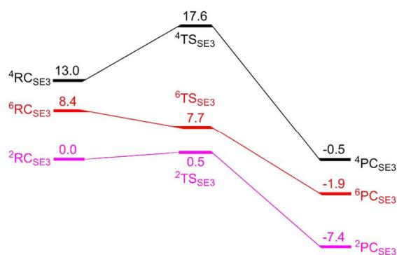
**Fig. 6** Energy profiles (in kcal/mol) for the reduction of  $\cdot\text{CCl}_3$  via a  $\text{S}_{\text{E}3}$  mechanism calculated at the UB3LYP/B2//B1 level on three spin states. All energy data include ZPE, solvation and dispersion corrections.
