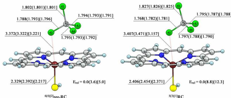
**Fig. 1** Geometries of the ferric- $\text{CCl}_4$  complex (pre-**RC**) and the ferrous- $\text{CCl}_4$  complex (**RC**) optimized at the UB3LYP/B1 level in the gas phase (bond distances indicated in Å) and the relative energies of various spin states (in kcal/mol) calculated at the UB3LYP/B2 level including zero-point energy (ZPE) and dispersion corrections.
