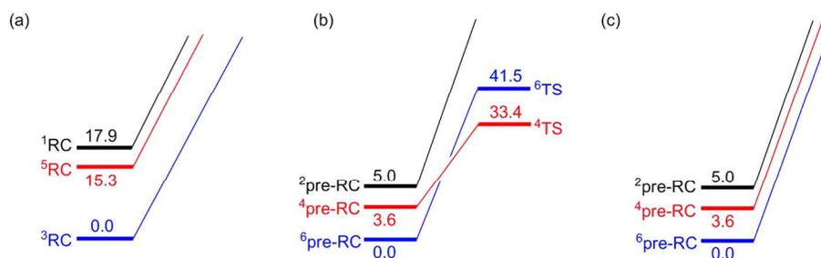
**Fig. 4** Scan energy profiles (in kcal/mol) at the UB3LYP/B1 level in the gas phase for the activation of (a) C-Cl<sub>distal</sub> bond by the ferrous haem complex; (b) C-Cl<sub>proximal</sub> bond by the ferric haem complex; (c) C-Cl<sub>distal</sub> bond by the ferric haem complex.
