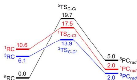
**Fig. 2** Energy profiles (in kcal/mol) for the initial reduction of  $\text{CCl}_4$  calculated with UB3LYP/B2//B1 on three spin states. All energy data include ZPE, solvation and dispersion corrections.
