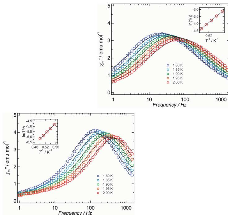
**Fig. 9**  $\chi''$  for the ladder complex, before (top) and after (bottom) irradiation by visible light, under a 1 kOe external dc field and a 3 Oe ac field. Inset is the Arrhenius plot of relaxation time. Adapted from ref 41
