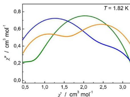
**Fig. 1** A comparison of the best fits of the Cole–Cole plots generated by using the Debye model for initial (orange), dry (blue), and rehydrated (olive) Dy SIMs at 1.82 K. Reproduced from Ref [17]
