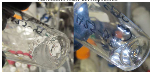
Fig. 1. 1:1 blend of AB:E before H 2 release (left) and after extended heating (right)
