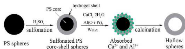
Figure 12. Diagram of the formation mechanism of the \text{CaO}/\text{Ca}_{12}\text{Al}_{14}\text{O}_{33} hollowspheres.
