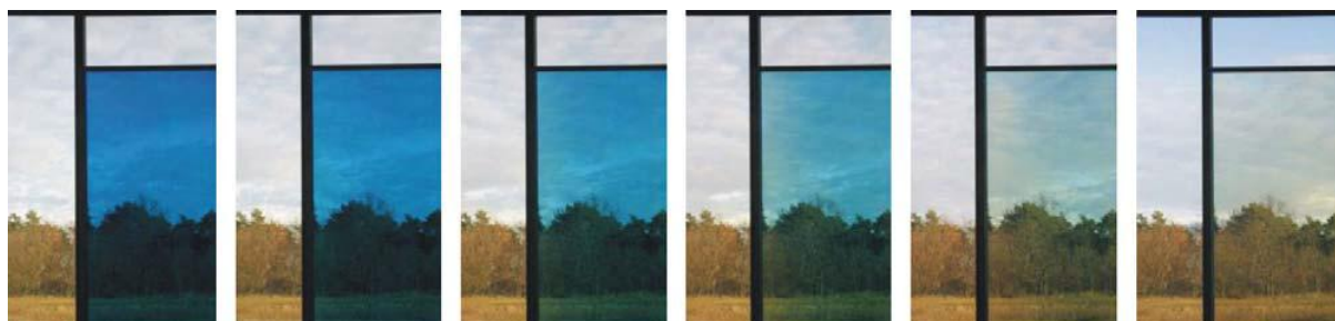
Figure 7: Switching sequence of an ECW. Figure adapted from reference 75 .
