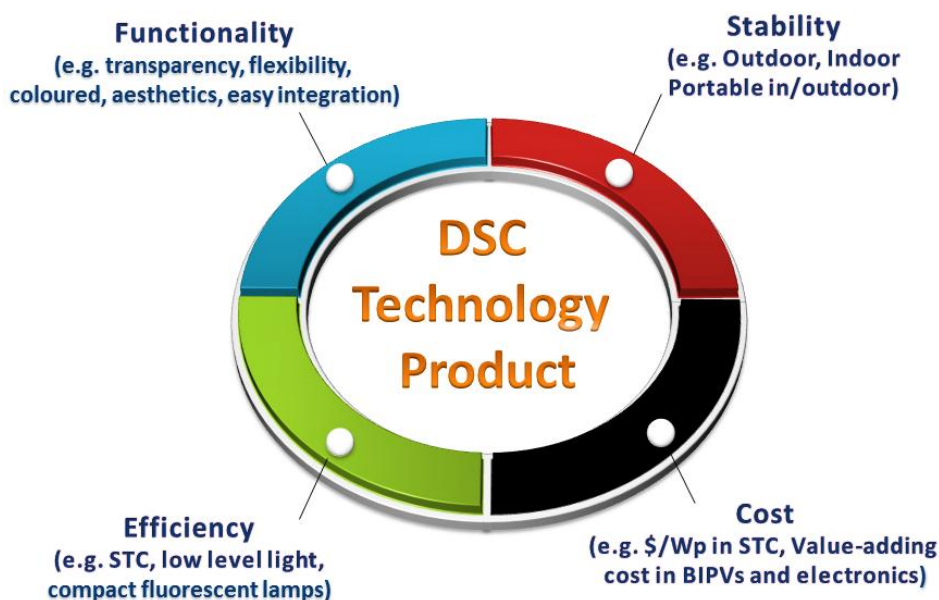
Figure 17: Scheme representing inter-relations between the three parameters (power conversion efficiency, stability and cost) which must be considered, together with functionality, for a successful industrial product development for dye solar cell modules. Different applications and markets lead to different mix of requirements and thus different DSM technological development (e.g. glass, flexible, material combinations, device architecturesetc).
