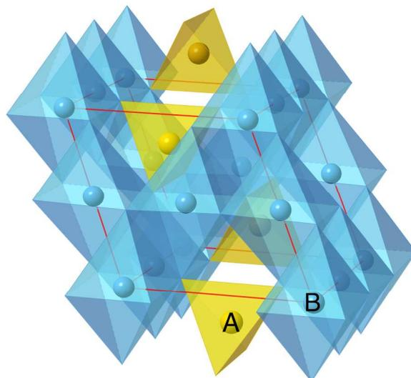
Fig. 1. The spinel crystal structure where the 'A' atoms occupy the tetrahedral sites, and the 'B' atoms occupy the octahedral site. Throughout this paper, the 'A' atoms are multivalent intercalating ions selected from the set  $\{\text{Mg}^{2+}, \text{Ca}^{2+}, \text{Zn}^{2+}, \text{Y}^{3+}, \text{Al}^{3+}\}$ , and the 'B' atoms are transition redox-active ions, selected from the set  $\{\text{Ti}, \text{V}, \text{Cr}, \text{Mn}, \text{Fe}, \text{Co}, \text{Ni}\}$ .
