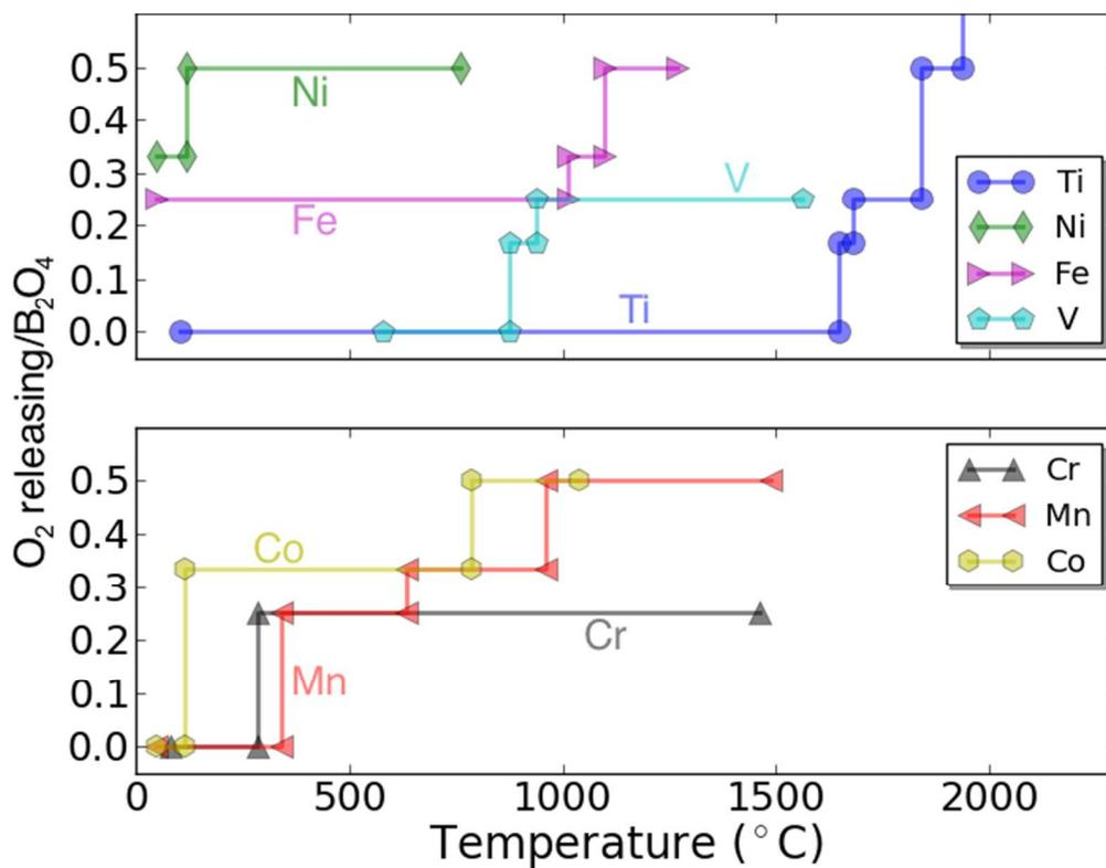
Fig 6. The calculated thermodynamic O<sub>2</sub> evolution diagram of charged host spinel compounds as a function of temperature. The vertical axis denotes how much O<sub>2</sub> is predicted to be released from the compound per formula unit of B<sub>2</sub>O<sub>4</sub> as the material decomposes.
