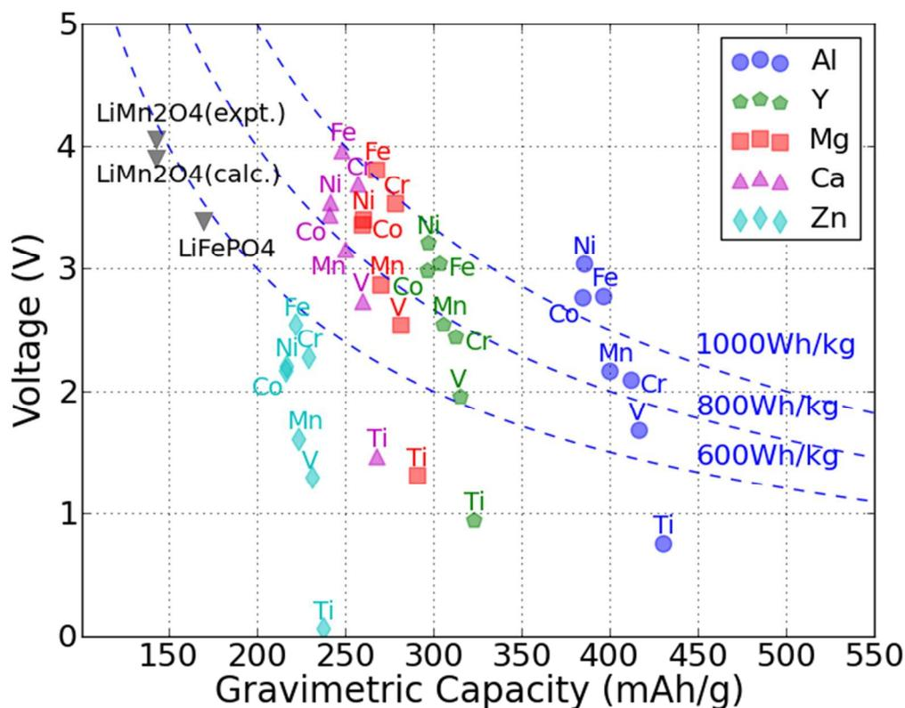
Fig. 2. The computed average voltage vs. gravimetric capacity for intercalation of A = Zn, Ca, Mg, Y and Al in various  $\text{M}_2\text{O}_4$  spinels up to composition  $\text{AM}_2\text{O}_4$ . The redox-active metal is marked next to each point. Dashed curves show the specific energy of 600Wh/kg, 800Wh/kg and 1000Wh/kg, respectively. The spinel  $\text{LiMn}_2\text{O}_4$  and olivine  $\text{LiFePO}_4$  data points are also marked on the plot for comparison<sup>22,36,43</sup>.
