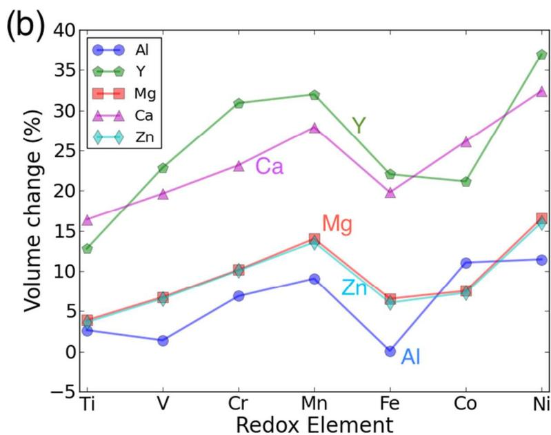
Fig. 4 The calculated (a) volumetric multivalent capacity and (b) volume change of the spinel structure as a function of the redox-active cation, assuming intercalation to composition  $AB_2O_4$ .
