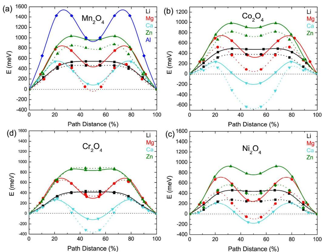
Fig. 7 Computed minimum energy paths for migration of different intercalants between the tetrahedral sites in the spinel  $B_2O_4$  ( $B = Mn, Co, Ni, Cr$ ) at the high vacancy limit (solid line) and dilute vacancy limit (dotted line), i.e. one mobile specie per supercell ( $2 \times 2 \times 1$  of primitive cell).
