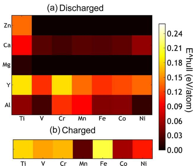
Fig. 5 a) The calculated thermodynamic stability of the  $AB_2O_4$  spinel compounds as a function of the intercalating ion (vertical axis) and redox metal (horizontal axis).
