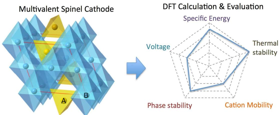
A matrix of spinel structures are systematically calculated and evaluated to screen for the improved multivalent battery cathode.
