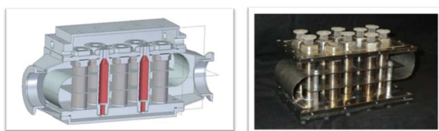
Fig. 5 Hydrogen release unit (HRU) consisting of ten parallel reactors mounted in vertical direction. Left: Schematic view showing the reactors in the hot air box – hot air enters the box from the left to ensure counter-current heat transfer; Right: Photograph of the open HRU unit with ten SEBM-manufactured and catalytically functionalized reactor tubes. The unit is surrounded by a box to guide the hot air flow.
