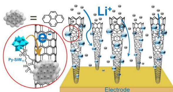
Figure 11. Schematic illustration of the Py-PW 11 /SWNTs/nanocomposite as anode material covalently functionalized POM clusters were attached to the SWNTs through \pi - \pi stacking interactions. 29
