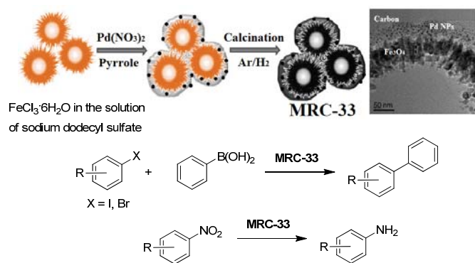
Fig.32 The schematic preparation of MRC-33 , the catalytic Suzuki reactions and the catalytic reductions.
