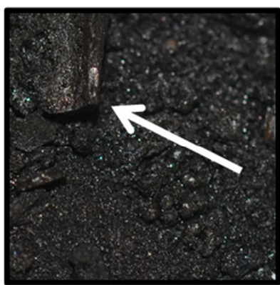
Figure 8: Large char agglomerate resulting from fast pyrolysis of AAEM passivated red oak.
