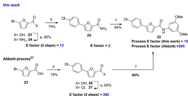
**Scheme 3.** Synthetic routes for the preparation of **22**: Conventional literature procedure vs green procedure.
