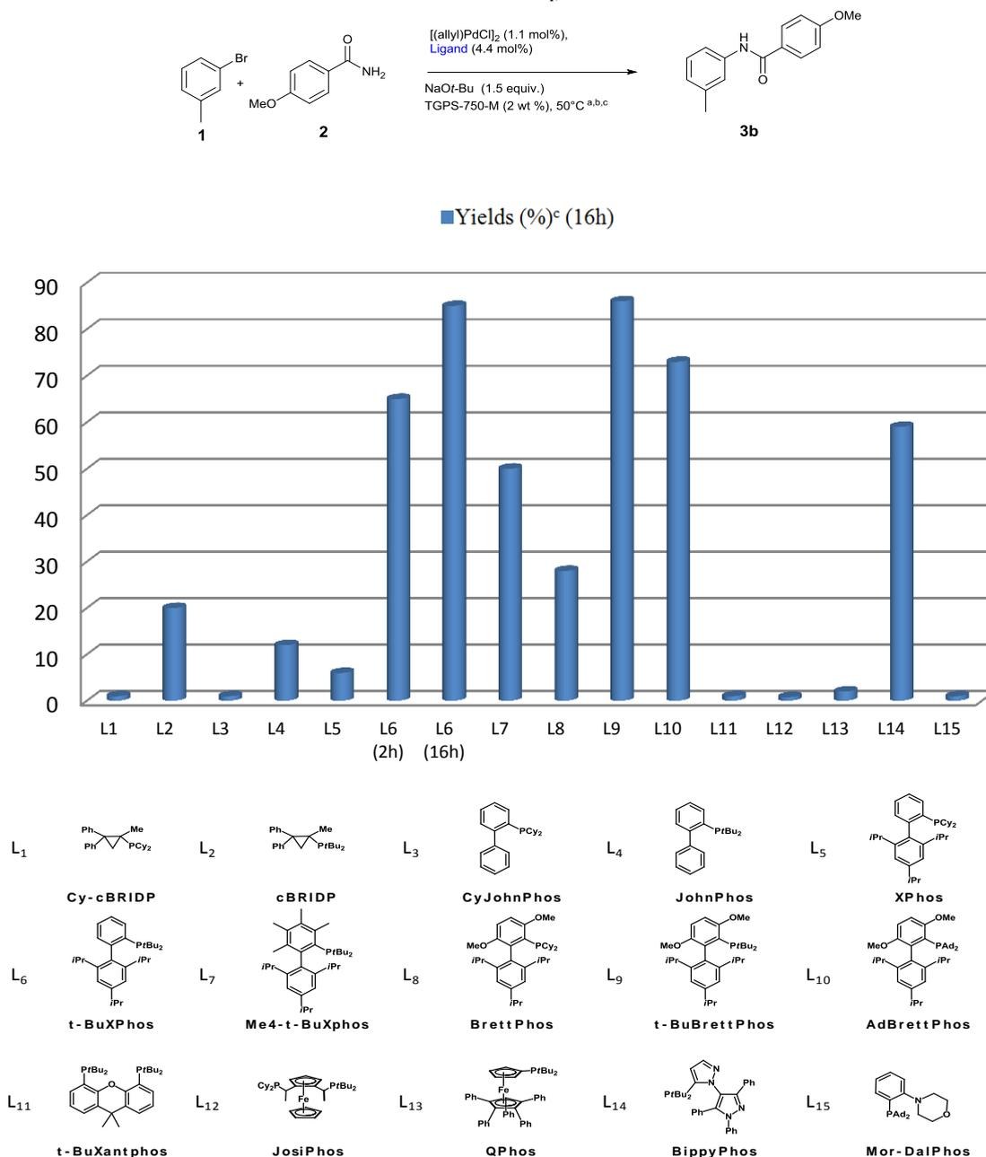
**Figure 1** Impact of various ligands on the efficiency of the aryl amidation reaction in TPGS -750-M.
