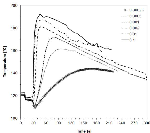
**Fig. 4** Effect of  $\text{Fe}(\text{acac})_3$  concentration (mol%; catalyst per hydroxyl) on exotherm profiles. Sequential addition of BDO/catalyst (80 °C) and  $\text{H}_{12}\text{MDI}$  (80 °C) to PTMEG-1000 (120 °C) under stirring (400 rpm).
