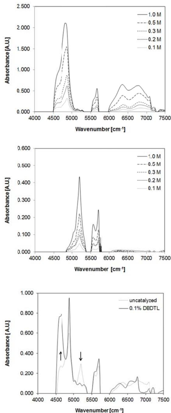
**Fig. 1** NIR spectroscopy for monitoring urethane formation from of 1-butanol and H<sub>12</sub>MDI. (a) concentration series (0.1 – 1 M) for 1-butanol; (b) concentration series (0.1 – 1 M) for H<sub>12</sub>MDI; (c) reaction mixture in the absence of a catalyst (dotted line) and reaction mixture containing 0.1 mol% of DBTDL as a catalyst. Peaks that are diagnostic for urethane formation and isocyanate consumption are marked.
