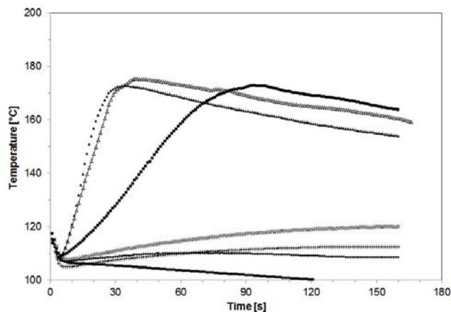
**Fig. 5** Effect of catalyst on exotherm profile, at 0.001 mol% catalyst on total hydroxyl basis. DBTDL (◆); UL-22 (■); Fe(acac)<sub>3</sub> (▲); Mn(acac)<sub>2</sub> (×); Hf(acac)<sub>4</sub> (+); Zr(acac)<sub>4</sub> (●); FeCl<sub>3</sub> (-△). Sequential addition of BDO/catalyst (80 °C) and H<sub>12</sub>MDI (80 °C) to PTMEG-1000 (120 °C).
