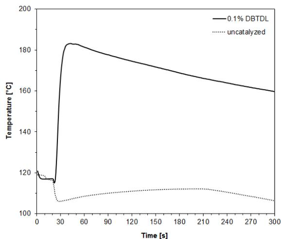
**Fig. 2** Exotherm profiles of uncatalyzed vs. catalyzed (0.1 mol% DBTDL) reaction mixtures. Sequential addition of BDO/catalyst (80 °C) and  $\text{H}_{12}\text{MDI}$  (80 °C) to PTMEG-1000 (120 °C) under constant stirring (400 rpm).
