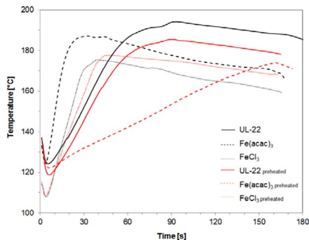
**Fig. 6** Effect of preheating on catalytic activity of UL-22 (full line), Fe(acac)<sub>3</sub> (dashed line) and FeCl<sub>3</sub> (dotted line). Sequential addition of BDO/catalyst (80 °C) and H<sub>12</sub>MDI (80 °C) to PTMEG-1000 (120 °C). Catalyst concentration of 0.001 mol%.
