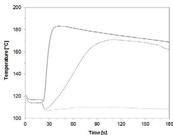
**Fig. 3** Effect of DBTDL concentration on exotherm profile: 0.1 mol% (full); 0.01 mol% (dashed) and 0.001 mol% (dotted). Sequential addition of BDO/catalyst (80 °C) and  $\text{H}_{12}\text{MDI}$  (80 °C) to PTMEG-1000 (120 °C) under constant stirring (400 rpm).
