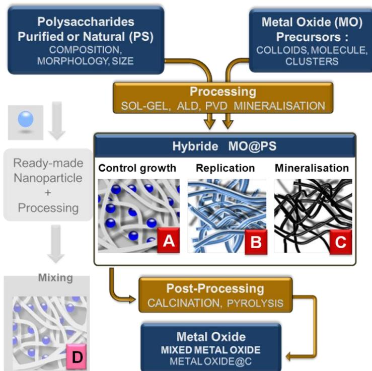
**Fig.3** A general overview of the different approaches in which PSs are introduced as biotemplate for the preparation of MO@PS, the latter being an intermediate leading, after PS removal, to MO. Alternatively pyrolysis in inert atmosphere lead to MO@C composite
