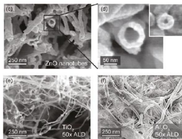
**Fig. 13** SEM images of ZnO@NCA (c,d);  $\text{TiO}_2$ @NCA (e) and  $\text{Al}_2\text{O}_3$ @NCA (f) obtained reactive ALD with nanocellulose aerogel.<sup>262</sup>
