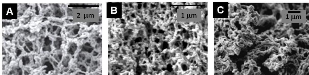
**Fig. 9** SEM images of different metal oxide nanoparticles assembled with different PS A : TiO<sub>2</sub>@Chitosan (20% acetylation),<sup>157</sup> B : TiO<sub>2</sub> after calcination of TiO<sub>2</sub>@Agarose composite;<sup>158</sup> C : YBa<sub>2</sub>Cu<sub>3</sub>O<sub>7</sub>@Dextran;<sup>159</sup>
