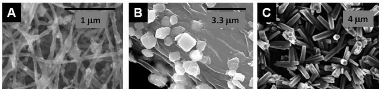
**Fig. 7** SEM images of examples of different metal oxide nanoparticles assembled with or produced from cellulose-type PS **A** : Fe<sub>3</sub>O<sub>4</sub>@BNC (from *Acetobacter xylinum*);<sup>122</sup> **B** : BiVO<sub>4</sub>@Cellulose (from *Eucalyptus globulus* wood cellulose fibres);<sup>123</sup> **C** : ZnO@Cellulose layer (from filter paper)<sup>124</sup>
