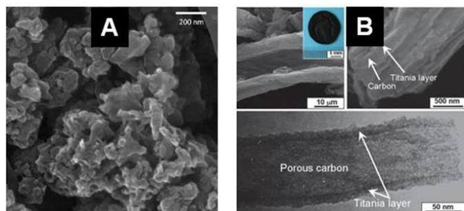
**Fig. 6** SEM (A) and TEM (B) images of example of an MO@C composite obtained by pyrolytic treatment of the corresponding hybrid MO@PS **A** : LiFePO<sub>4</sub>@C from filter paper after impregnation with (LiNO<sub>3</sub>/FeSO<sub>4</sub>) and pyrolysis under Ar+H<sub>2</sub><sup>117</sup> **B** : TiO<sub>2</sub>@C from ashless filter paper impregnated with TTB and pyrolysis under N<sub>2</sub>.<sup>118</sup>
