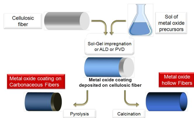
**Fig. 10** General pathway for metal oxide preparation by impregnation/deposition with PS, leading to hybrids  $M_xO_y@PS$  and then  $M_xO_y$  or  $M_xO_y@C$  material upon thermal treatment.
