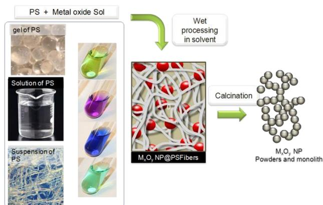
**Fig. 4** The general pathway for the control of the growth of MO nanoparticles by the presence of PS
