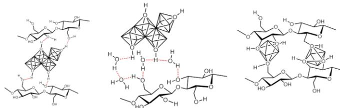
**Fig. 5** Schematic representation of the possible interaction between functions of polysaccharide units and metal-containing species
