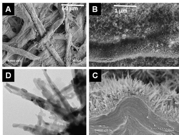
**Fig. 14** SEM (A, B, C) and TEM (D) picture of  $\text{TiO}_2@$  filter paper obtained by mineralization of filter paper by  $\text{TiCl}_4$  in anhydrous condition at  $80^\circ\text{C}$ .<sup>3</sup>
