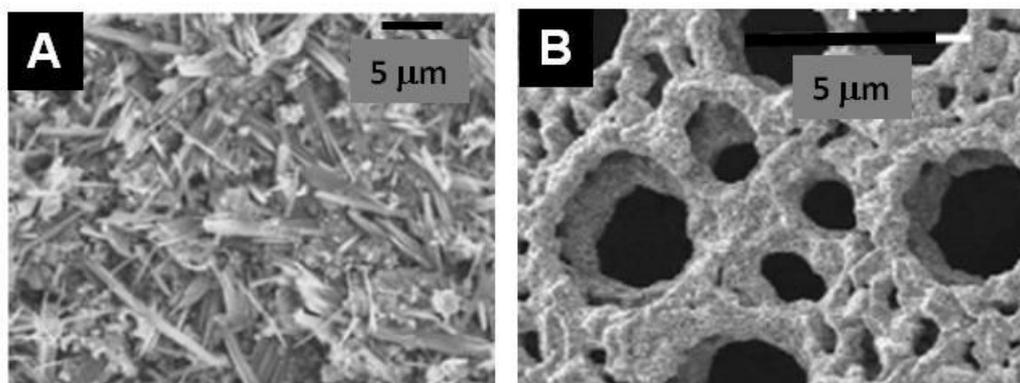
**Fig. 8** SEM images of examples of different metal oxide nanoparticles assembled with or produced from alginate-type PS. A : La<sub>0.67</sub>Sr<sub>0.33</sub>MnO<sub>3</sub> with sodium alginate;<sup>140</sup> B : CuO after calcination of Cu-alginate aerogel from sodium alginate.<sup>138</sup>
