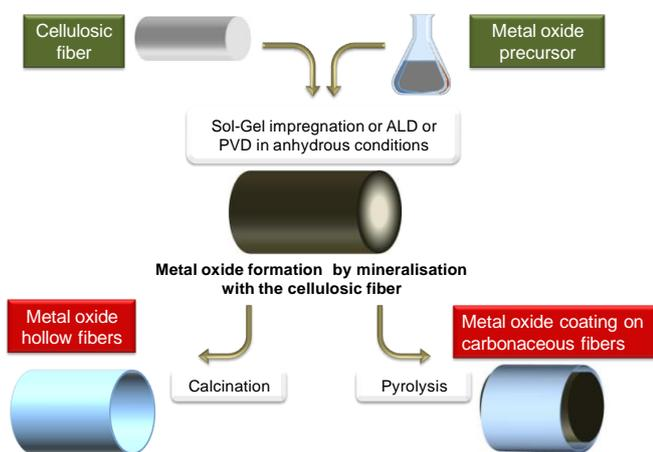
**Fig.12** General scheme of the polysaccharide mineralisation process leading to hybrid  $M_xO_y$ @PS and then to either  $M_xO_y$  or  $M_xO_y$ @C materials
