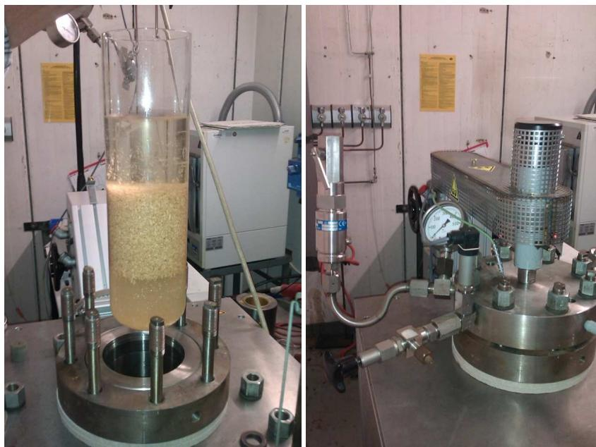
**Figure 1.** Reaction-setup at 3 L scale. Left: Filled glass inlay with substrate, catalyst and solvents; Right: Closed high pressure reactor.
