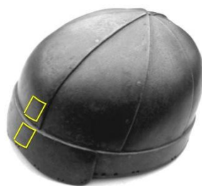
Fig 4: Picture indicating the measuring points (circa 2.5 \times 2.5 \text{ cm}^2 ) for the INES diffraction measurement.
