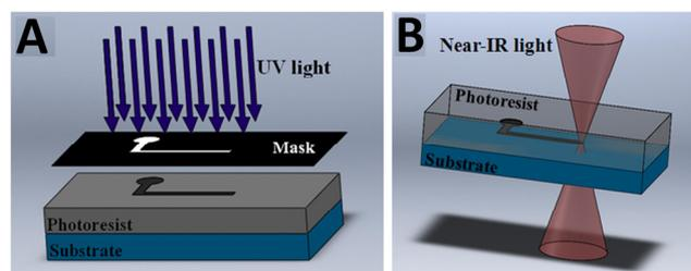
**Fig. 2** Two different approaches to the polymerization of a negative photoresist. (A) Conventional UV lithography, where light is projected through a shadow mask onto a photosensitive material. (B) Two-photon polymerization: High resolution 3-D structures are written in the volume of the photoresist using a pulsed near-IR laser.
