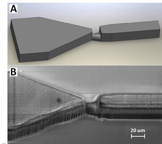
**Fig. 3** (A). CAD image of the 3-D structure that traps *J2 G. pallida*. (B) SEM image of the semi-cylindrical trapping channel. The rounded shape (written with the Nanoscribe) provides a tight fit to the contours of the worm.
