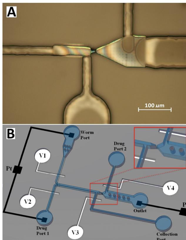
**Fig. 4** (A) Photograph of the SU-8 master that is used to fabricate the StyletChip. (B) Schematic layout of the chip showing the integrated Pt electrodes (at inlet and outlet), the trap region (inset) and the four valves (V1, V2, V3 and V4) used to control worm loading (V1), chemical or drug delivery (V2 and V4) and worm retrieval (V3).
