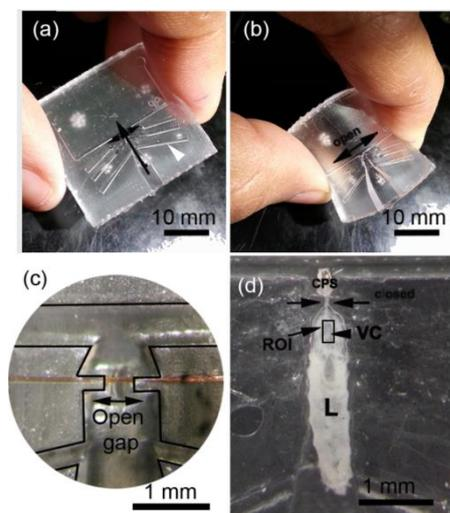
Fig. 6: Steps to load the larva using the FlexiChip. The chip is bent (b) so that the clip (c) opens. Then, the animal is inserted into the gap and the chip is released and sealed by a coverslip (d). Time-lapsed fluorescent imaging was then conducted on the CNS located inside the Region of Interest (ROI)<sup>31</sup>
