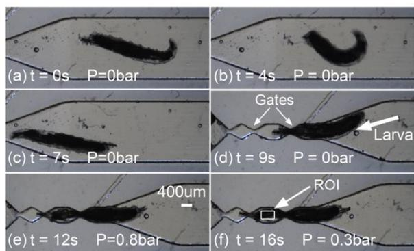
Fig. 5: Steps to load the larva using the pneumatic chip. (a-d) larva swam freely into the trap, (e-f) larva was pneumatically moved into the trap and immobilized. Time-lapsed fluorescent imaging was then conducted on the CNS located inside the Region of Interest (ROI). Scale bar=400  $\mu\text{m}$  for all figures is shown in Fig. 5e.
