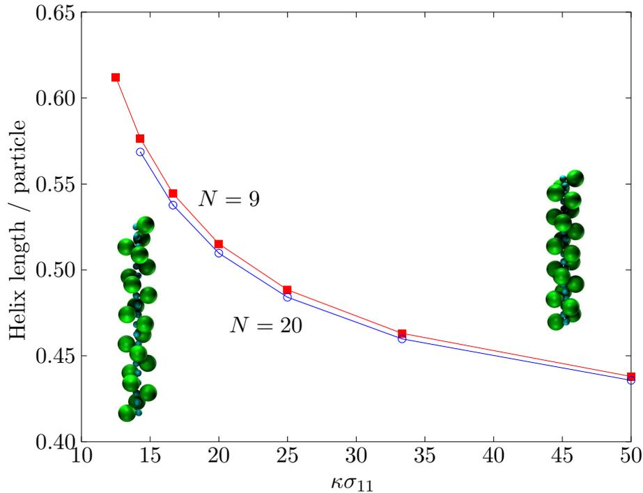
FIG. 2: Helix length per particle as a function of the inverse screening length for the predicted ground state structures. Results are shown for  $N = 9$  and  $N = 20$ . Insets: the ( $N = 20$ ) helix configurations for (left)  $\kappa\sigma_{11} = 14.3$  and (right)  $\kappa\sigma_{11} = 50.0$ . The dipoles are not shown for clarity of presentation.
