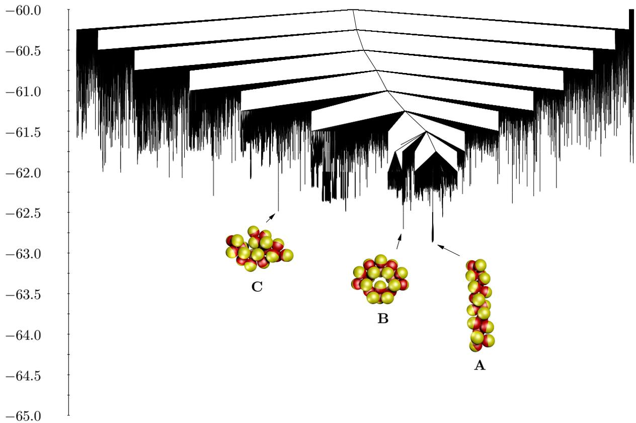
FIG. 5: Disconnectivity graph for  $N = 20$  Janus building blocks. The global minimum is a Bernal spiral (**A**), which is very flexible. In this graph, more than 30 minima around the global minimum exhibit bent structures, which interconvert *via* ‘hinge’ motions. The lowest energy kinetic trap (**B**) corresponds to a symmetric cyclic structure, while the second-lowest (**C**) is a dimer of a low-energy minimum for  $N = 10$ .
