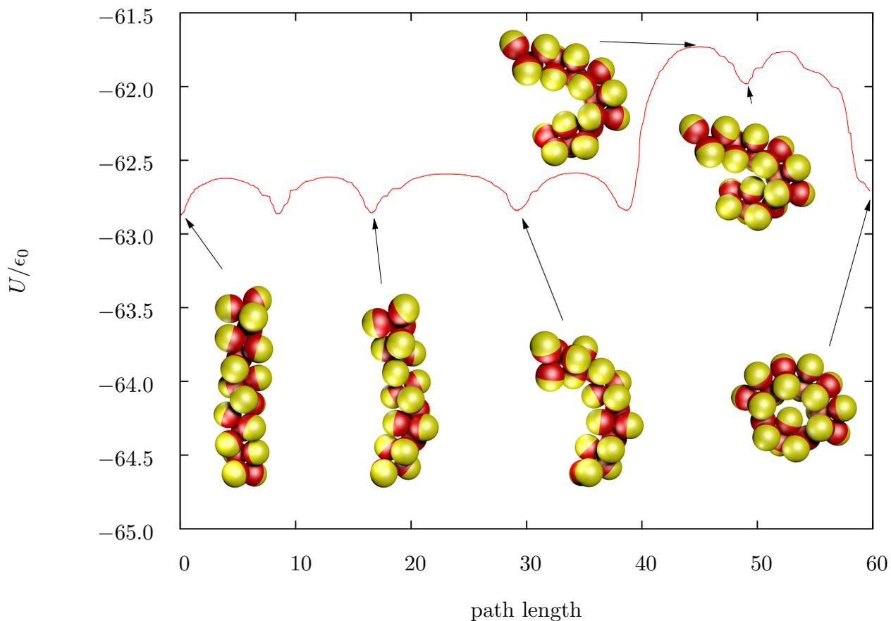
FIG. 7: Fastest pathway between the tetrahelix global minimum and a low-energy closed ring structure. The rearrangements with energy barriers of about  $0.25 \epsilon_0$  are all ‘hinge’-motions. Structures for selected minima and the highest energy transition state are also shown.
