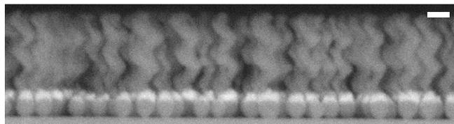
**Fig. 12** SEM cross-section image of small magnetic swimmers. Contrast in image clearly shows location of magnetic Ni section (light color). Scale bar 100 nm.
